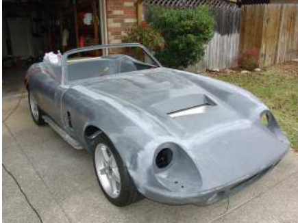
First rough sanding process on the body.
