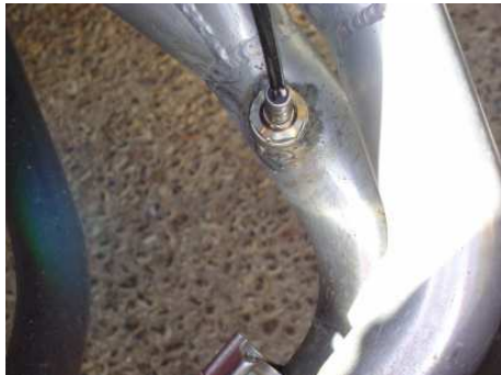
Passenger side O2 sensor and location
