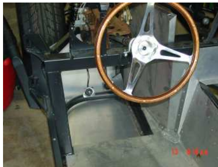
Center front panel attached to driver floor / foot box.
