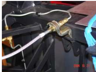
Rear brake line to flexible mount showing steel line and flexible connection assembly.
