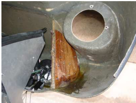
Hood rib panel with fiberglass and wood strengthening applied
