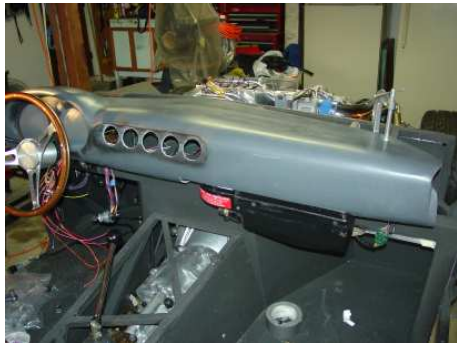
First dash fitting to determine AC space behind it
