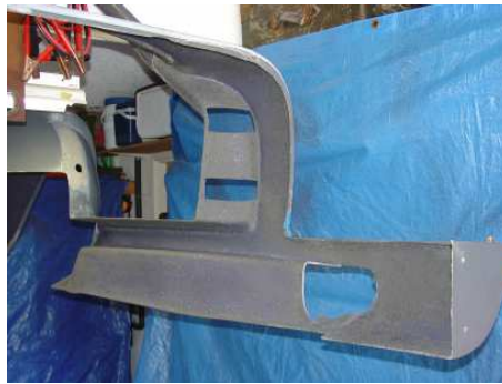
Driver body under side showing Lizard Skin shield
