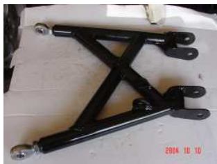
Lower IRS Control Arm with rod ends.
