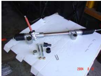
Flaming River steering rack assembly with bushings and frame installation bolts.
