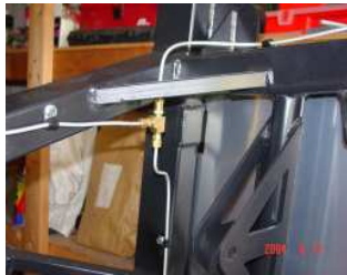
Main rear steel brake line, tee for driver and passenger side fittings.
