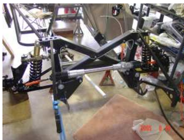
Final IFS suspension assembly installed and torqued with front and back views.
