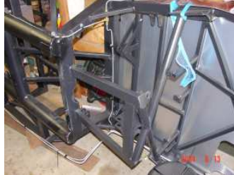
Driver side attachment points for control arms, quad-shocks and coil-over shocks.
