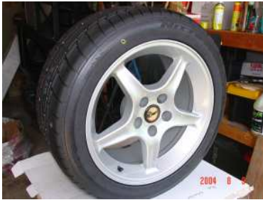
Cobra R Silver 17 x 9 five lug wheel with 245 45 ZR 17 Nitto tires for front.
