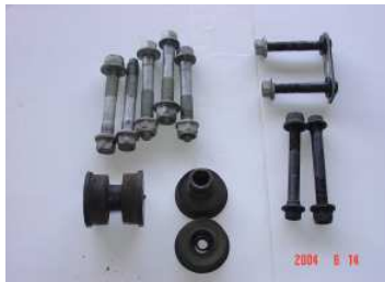
Ford bolts and nuts to save along with the front differential mounts. Note that one spindle bolt and two nuts were lost in shipment.
