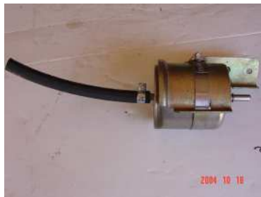
Fuel filter bracket and fuel filter lay out before installation. Fuel Filter bracket after modification.
