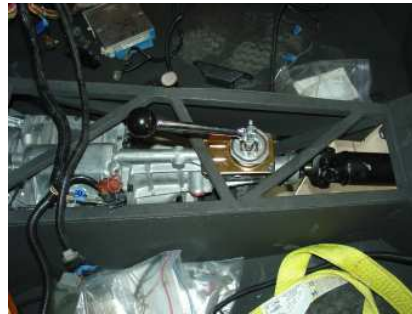
Drive train, including drive shaft installed in chassis
