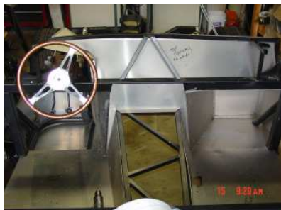
Driver center front tunnel panel attached to footbox.
