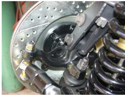
Passenger spindle with raised tie rod arm.
