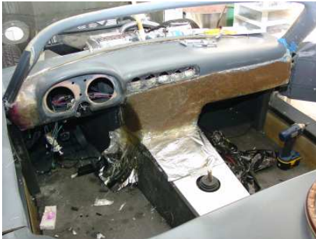
Fiberglass Bondo for thickness buildup
