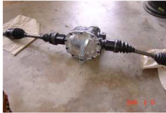
Two views of the 8.8 Thunderbird Supercoupe Traction-Lok differential with the FFR half-shafts and Boots installed.
