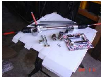
Flaming River steering rack assembly with bushings and frame installation bolts.
