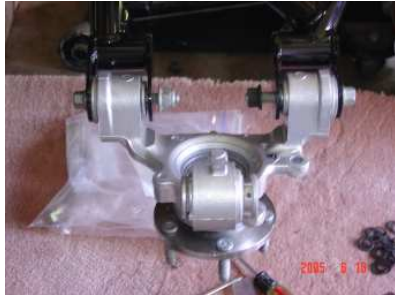
Driver side spindle attached to lower control arm brackets.
