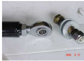
Rod end assembled with bolt parts.
