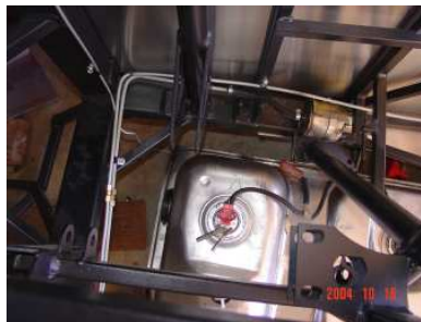
Fuel line routed to the fuel filter installed on the passenger side frame. View of fuel filter mounted before gas tank installed. Fuel return line mounted close by the fuel line.
