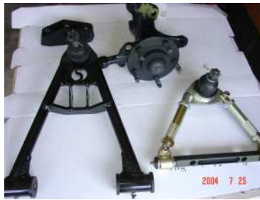
Major front suspension components, upper and lower control arm, Mustang spindle, IFS bracket, and Baer five lug spindle hub.
