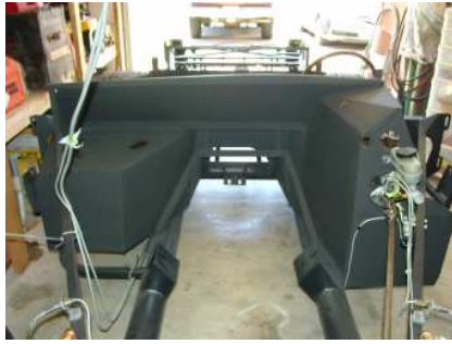
Firewall after LizardSkin application.
