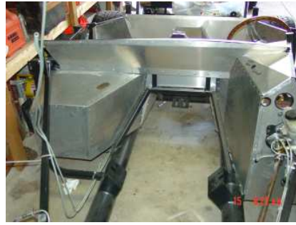
Firewall after assembly with pop rivets.
