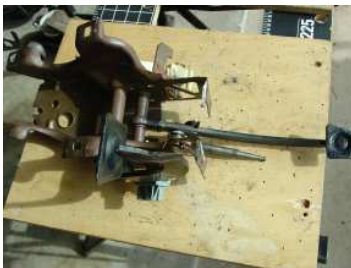
The modified brake pedal installed in the pedal box assembly.
