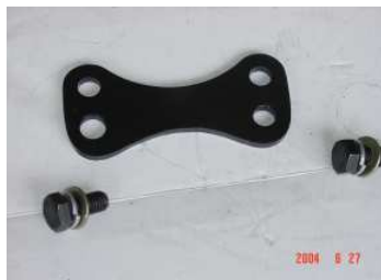
AMP spindle to caliper plate with spindle bolts
