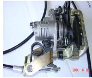
Emergency brake cable in the attachment point and connected to the caliper lever.
