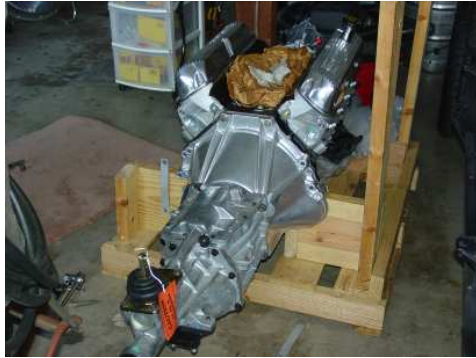
Drive train assembly on engine before install
