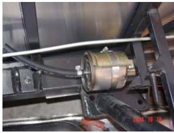
Fuel filter and bracket mounted on passenger side of the frame at the end of the 3" x 2" frame tube.
