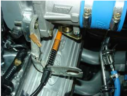
Throttle bracket to be shortened and temporally fitted.
