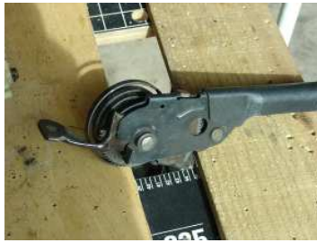
The emergency brake handle assembly as modified.
