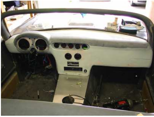
Modified dash with most of the holes cut into
