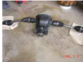
Two views of the 8.8 Thunderbird Supercoupe Traction-Lok differential with the FFR half-shafts and Boots installed.
