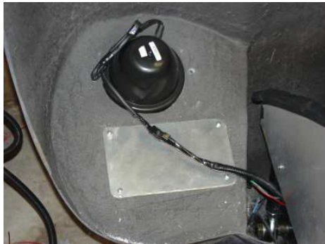
Nose body with Lizard Skin heat shield
