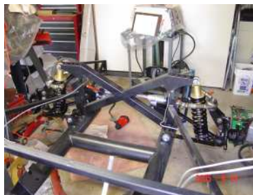
Final IFS suspension assembly installed and torqued with front and back views.
