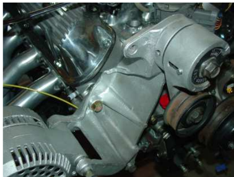
Bracket modification by grinding metal away
