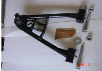
Front lower control arm with fittings and ball joint.
