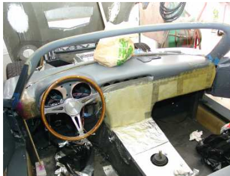
finished fiberglass mold ready with dash corners
