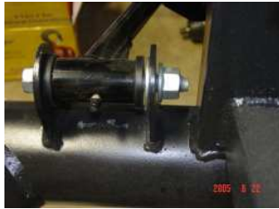
Driver side bracket at 1 \frac{7}{32} ".
