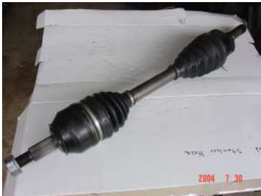
FFR half shaft with CV joints and FFR boots installed.
