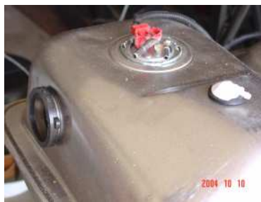
Close-up of the fuel 5/16 inch outlet and 1/4 inch return.
