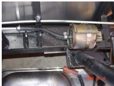
Fuel line routed to the fuel filter installed on the passenger side frame. View of fuel filter mounted before gas tank installed. Fuel return line mounted close by the fuel line.
