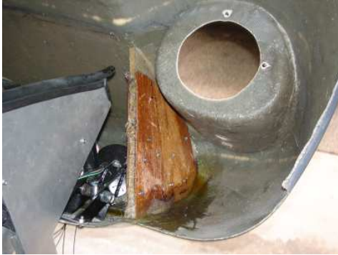
Passenger hood strut with ply and fiberglass
