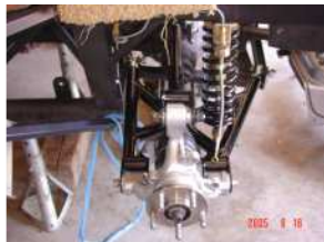
The shock/spring in place on the driver side IRS assembly.
