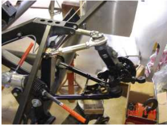
Driver side IFS assembly supported by jack.
