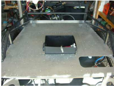
Trunk deck with battery well and box
