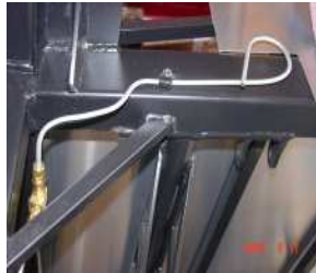
Main rear steel brake line, tee for driver and passenger side fittings.
