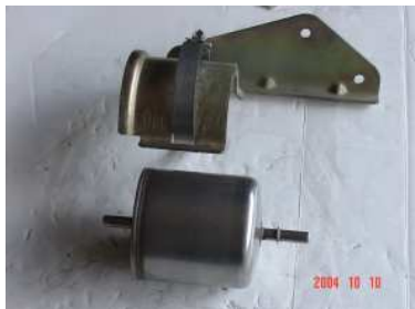
Fuel filter bracket and fuel filter lay out before installation. Fuel Filter bracket after modification.
