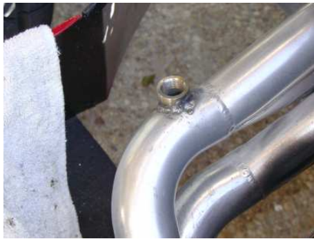
Bun welded into the driver side
