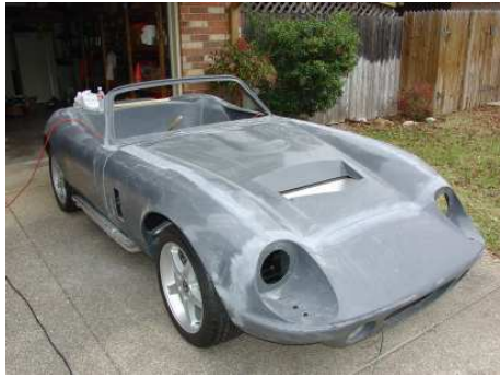
Body and hood after rough sanding of seams
