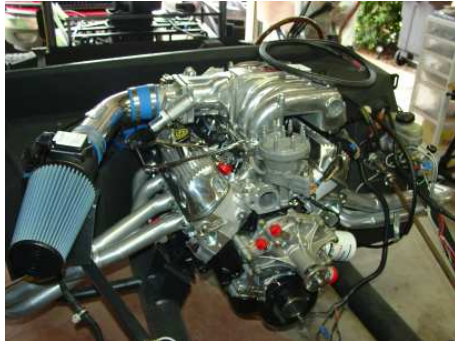
BBK throttle body, Mass Air sensor installed
