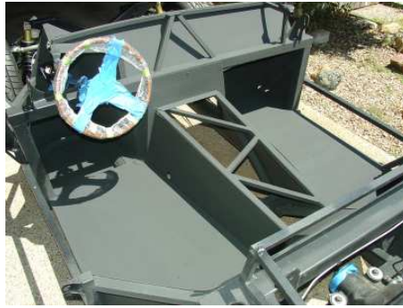
LizardSkin ceramic coating inside cockpit.
