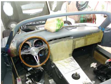
The mold for the AC cover and center console
