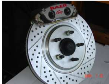
Baer thirteen inch slotted, drilled rotor.
