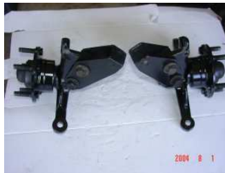
Pair Mustang spindles with FFR IFS strut brackets installed and torqued to 100 ft-lbs.
