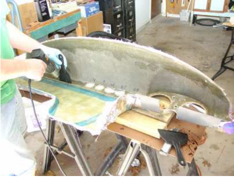
Laying the dash fiberglass in the mold we mfg
