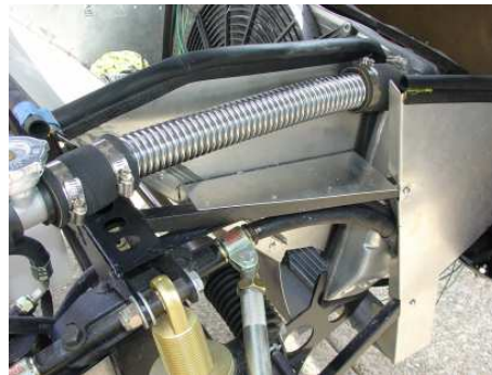
Air duct chassis brace attached to air duct and chassis. 180 minutes
