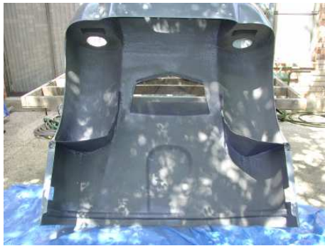
Nose body with Lizard Skin heat shield
