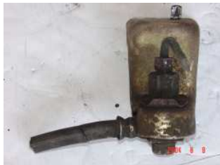
Mustang steel to flexible brake line mounts for rear mount.
