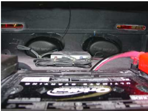
Trunk view of speakers and XM radio unit over battery
