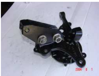
Mustang spindle with FFR IFS bracket installed.
