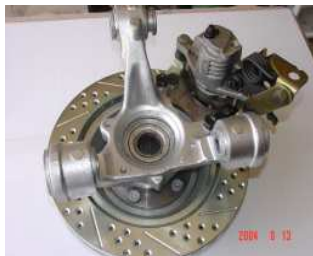
Baer assembly attached to T-bird spindle bolts.
