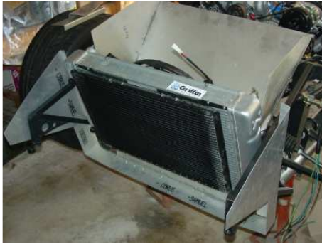
First fitting of air duct to radiator from front
