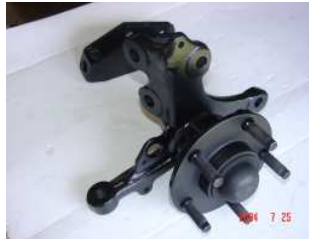
'96 Mustang spindle assembly with Baer five bolt hub end.
