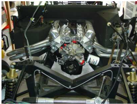
Engine with exhaust headers installed and lower intake manifold sitting in place
