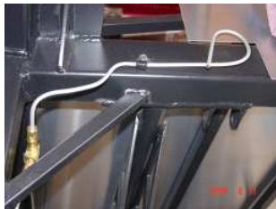
Rear brake line to flexible mount showing steel line and flexible connection assembly.
