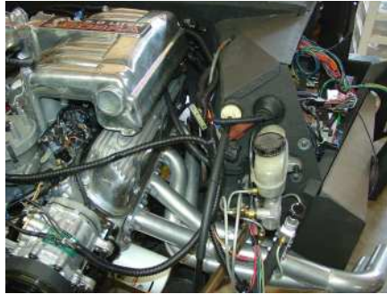
Clutch cable routed around headers
