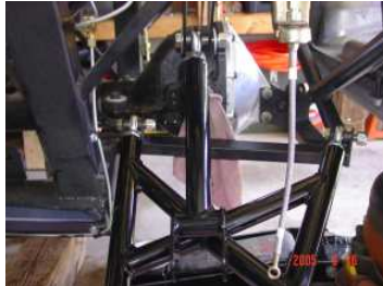
The upper IRS control arm located in the chassis bracket as it awaits installation in the hub assembly.
