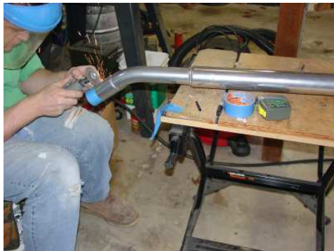
Photo of the exhaust as we cut it to length fit
